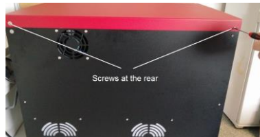
Remove two screws at the rear.
